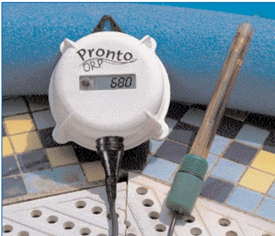
HI 982401 is a simple-to-operate, practical meter for ORP (Oxidation Reduction Potential) measurements. It continuously monitors ORP from -999 to +999 mV. Operators can also set the ORP level at which their application will produce the best results.
