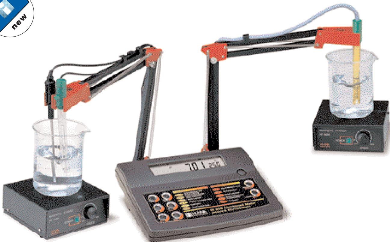
The new **HI 255** is the product of 26 years of instrument testing and design experience. It is the first laboratory bench meter to simultaneously perform precise, repeatable pH and conductivity measurements.
