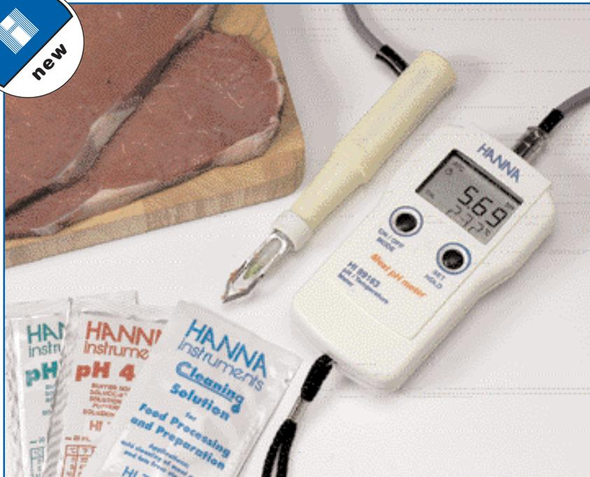
HI 99163 is a specific instrument for the pH analysis of meat products. The specially designed electrode FC 232D incorporates many essential features to perform reliably without damaging the sample. This probe has a built-in temperature sensor that provides automatic temperature compensation, an open junction to avoid a clogged reference and its external body material isn't toxic.
