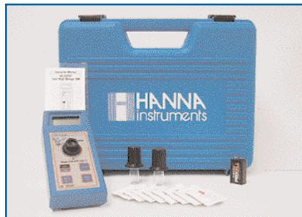
HI 93721C is the ideal solution for iron measurement in the field
