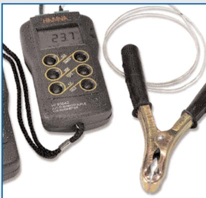
To partially solve this problem, **HANNA** instruments® has devised the calibration of the instrument-thermocouple system, by dipping the probe in melting ice, and thus allowing the user to calibrate the measuring system at 0°C. Thanks to this solution, it is now possible to use thermocouple thermometers for HACCP controls with an accuracy of  $\pm 0.3^\circ\text{C}$ , which is the same performance of our Pt100 or NTC thermometers, but with a higher response time.
