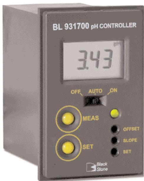
BL 931700 mini pH controller has been designed for easy, affordable installation in tight spaces to perform simple yet effective process control.
